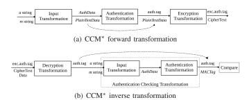
Figure 5: Block diagram of CCM\* mode of operation.
