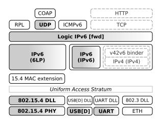
Figure 1: Communication stack architecture.
