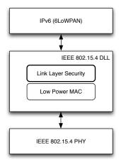
Figure 2: Link layer security module.
