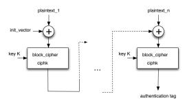
Figure 4: Diagram of the CBC-MAC mode of operation.
