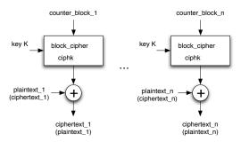
Figure 3: Diagram of the CTR encryption (decryption) mode.
