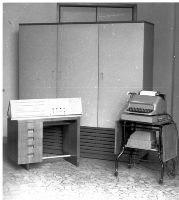
FIGURE 1. MS complete with control panel, left, and I/O peripherals, right. (Courtesy of Francesco Contin).
