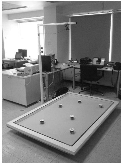
Fig. 1. Experimental setup consisting of an arena, robots, PC and overhead camera.
