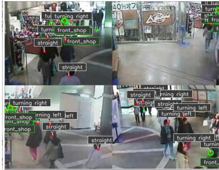
Fig. 7. Symbolic and numerical localization data measured in a shopping mall. The measurement is done by an environmental sensing system, and is provided to service robots.
