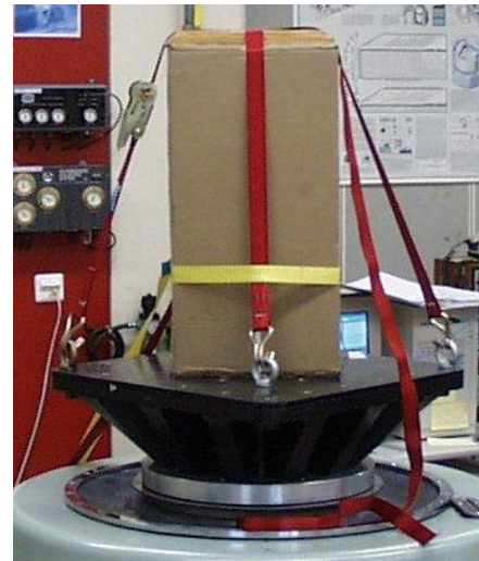
Fig. 19: Vibration test with IGCTs wrapped in transport box.
