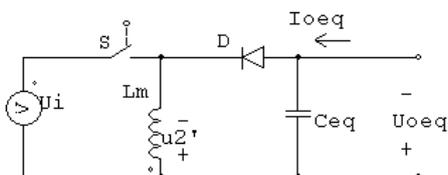
$$\text{dove: } C_p = \frac{2 \cdot C}{n^2} \quad I_{oeq} = \frac{I_o'}{n} + \frac{I_o''}{n} = \frac{0.5 + 0.5}{52.5} = 19 \text{mA} \quad U_{oeq} = 12 \cdot 52.5 = 630 \text{V}$$
