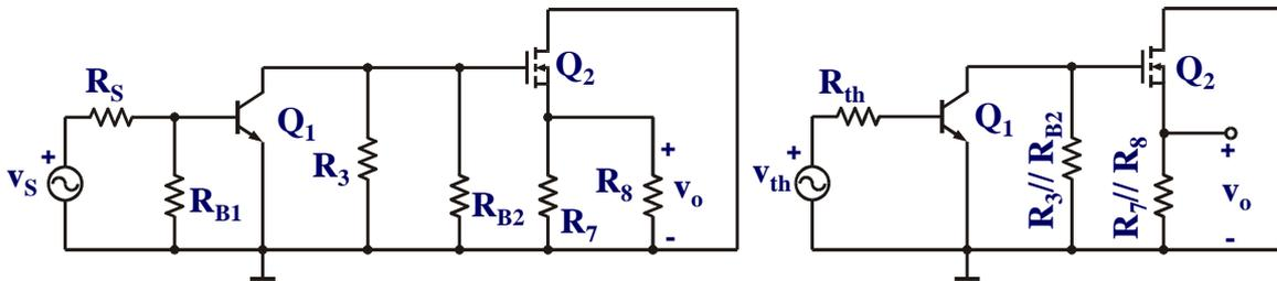
$$R_{B1} = R_1 // R_2 \quad R_{B2} = R_5 // R_6 \quad R_{th} = R_{B1} // R_S, \quad v_{th} = \frac{R_{B1}}{R_{B1} + R_S} v_s$$
