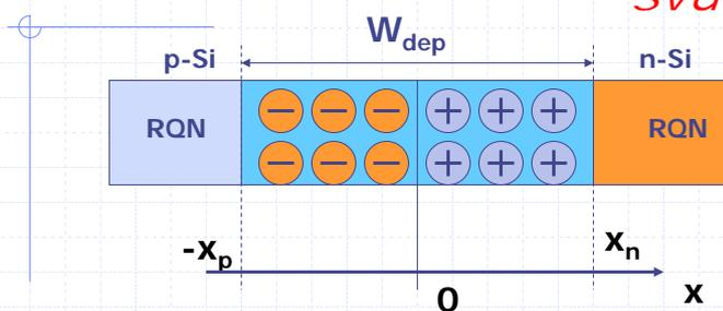
$$W_{\text{dep}} = x_p + x_n = \sqrt{\frac{2\varepsilon_s}{q} \left( \frac{1}{N_A} + \frac{1}{N_D} \right) V_0} \quad \frac{x_n}{x_p} = \frac{N_A}{N_D}$$
