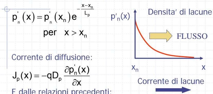
$$J_p(x) = q \frac{D_p}{L_p} p_{n0} \left( e^{\frac{V_A}{V_T}} - 1 \right) e^{-\frac{x-x_n}{L_p}} \quad \text{per } x > x_n$$
