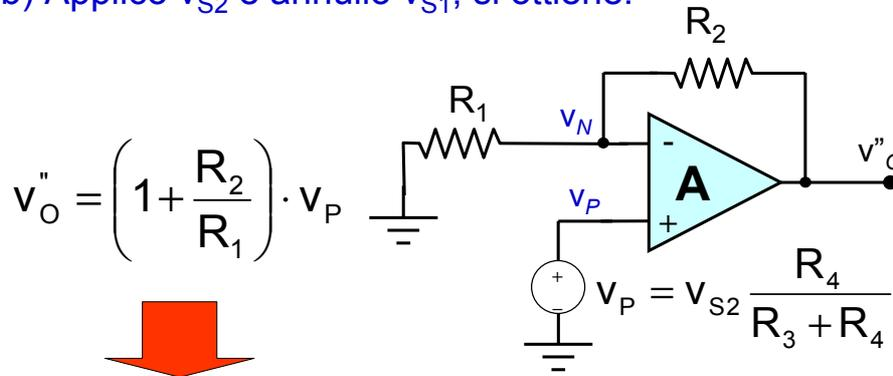
$$v''_O = v_{S2} \left( \frac{R_4}{R_3 + R_4} \right) \left( 1 + \frac{R_2}{R_1} \right)$$
