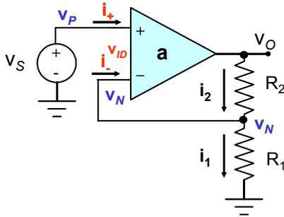
$$A_v = \frac{v_O}{v_S} = \frac{A}{1 + \frac{AR_1}{R_2 + R_1}} = \frac{A}{1 + A\beta}$$
