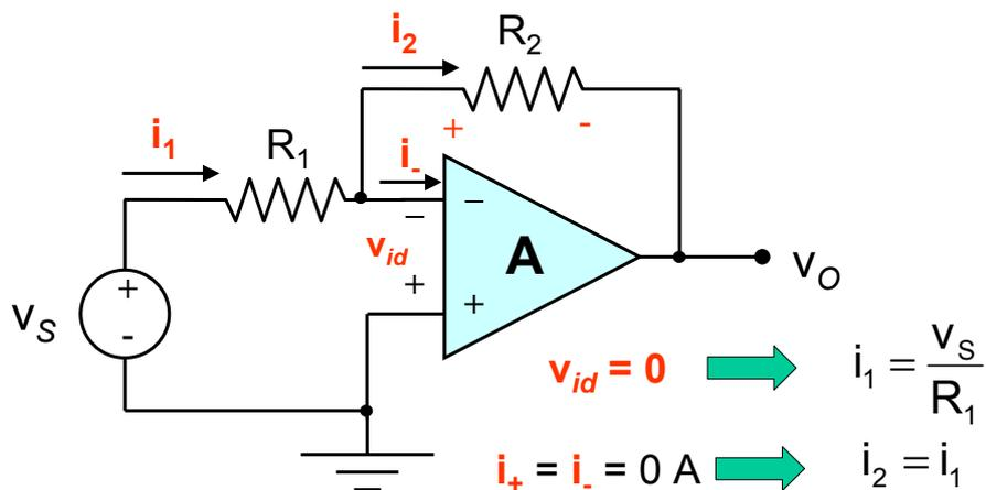
$$v_O = -R_2 i_2 = -\frac{R_2}{R_1} v_S$$
