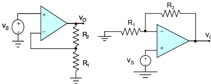
$$A = \frac{v_o}{v_s} = \left(1 + \frac{R_2}{R_1}\right)$$
