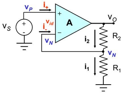
$$v_O = A \left( v_S - \frac{R_1}{R_2 + R_1} v_O \right)$$
