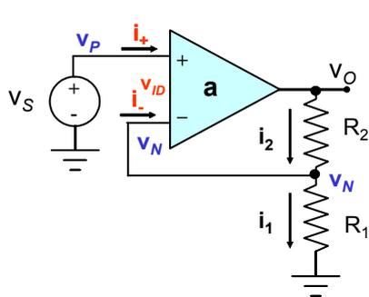
$$A_v(j\omega) = \frac{v_O}{v_S} = \frac{\frac{A_0 \omega_B}{\omega_B + j\omega}}{1 + \beta \frac{A_0 \omega_B}{\omega_B + j\omega}}$$
