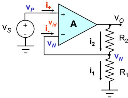
$$\lim_{a \rightarrow \infty} v_{id} = \lim_{a \rightarrow \infty} \frac{v_S}{1 + \frac{AR_1}{R_2 + R_1}} = 0$$
