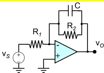
$$Z_2 = \frac{R_2 \cdot \frac{1}{sC}}{R_2 + \frac{1}{sC}} = \frac{R_2}{1 + sCR_2}$$
