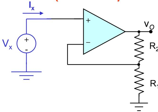
$$R_{IN} = \frac{V_x}{I_x} \quad \text{ma } I_x = 0 \quad \rightarrow \quad R_{IN} = \infty$$
