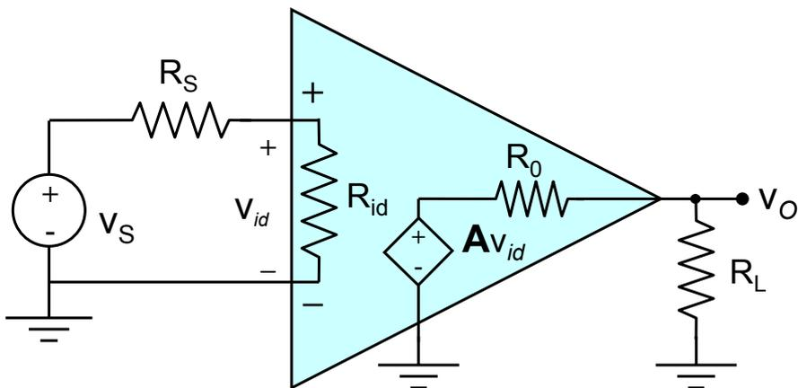
$$A_v = \frac{v_o}{v_s} = A \cdot \frac{R_{id}}{R_{id} + R_s} \cdot \frac{R_L}{R_L + R_0} < A$$
