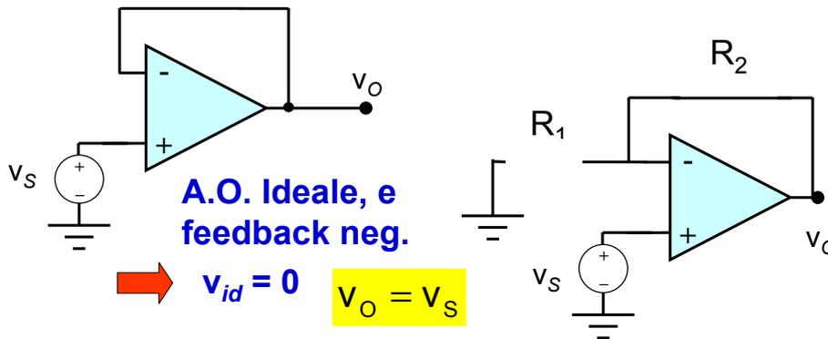
$$A_v = \frac{v_O}{v_{IN}} = \left(1 + \frac{R_2}{R_1}\right) \quad \Rightarrow \quad \begin{matrix} R_1 \rightarrow \infty \\ R_2 = 0 \end{matrix} \quad \Rightarrow \quad A_v = 1$$
