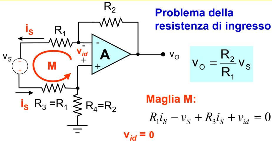
$$R_{id} = \frac{v_s}{i_s} = R_1 + R_3 = 2R_1$$
