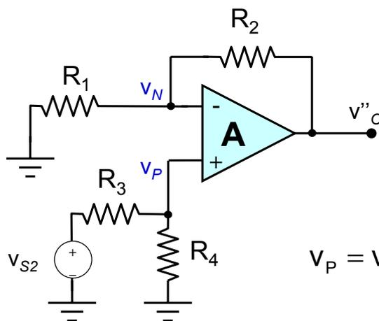
$$v_P = v_{S2} \frac{R_4}{R_3 + R_4}$$
