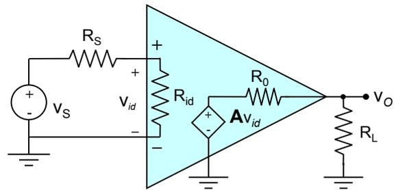
$$A_v = \frac{v_o}{v_s} = A \cdot \frac{R_{id}}{R_{id} + R_s} \cdot \frac{R_L}{R_L + R_0} < A$$
