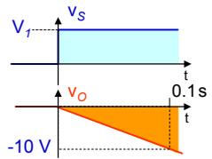
$$v_o(t) = \begin{cases} 0 & t < 0 \\ -\frac{V_1}{R_1 C_f} t & t \geq 0 \end{cases}$$
