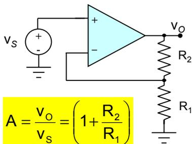
$$A = \frac{v_o}{v_s} = \left( 1 + \frac{R_2}{R_1} \right)$$
