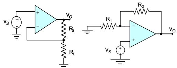
$$A = \frac{v_o}{v_s} = \left( 1 + \frac{R_2}{R_1} \right)$$
