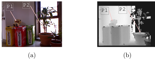
Figure 2: Example of kinect acquisition. Images show (a) color and (b) depth components. Corresponding points P1 and P2 are highlighted in the images related to bearbins .
