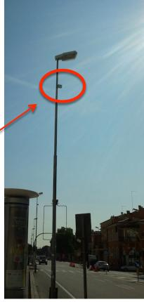
Sensor node protected by transparent plastic shield that permits air circulation
