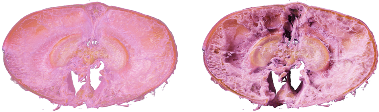
Figure 1: Example of benefits when applying global illumination to a fine-detailed volume visualization of micro CT scan of the insides of a fly head. Left: traditional diffuse illumination. Right: illumination through global illumination where fine structures appear much more clearly.
