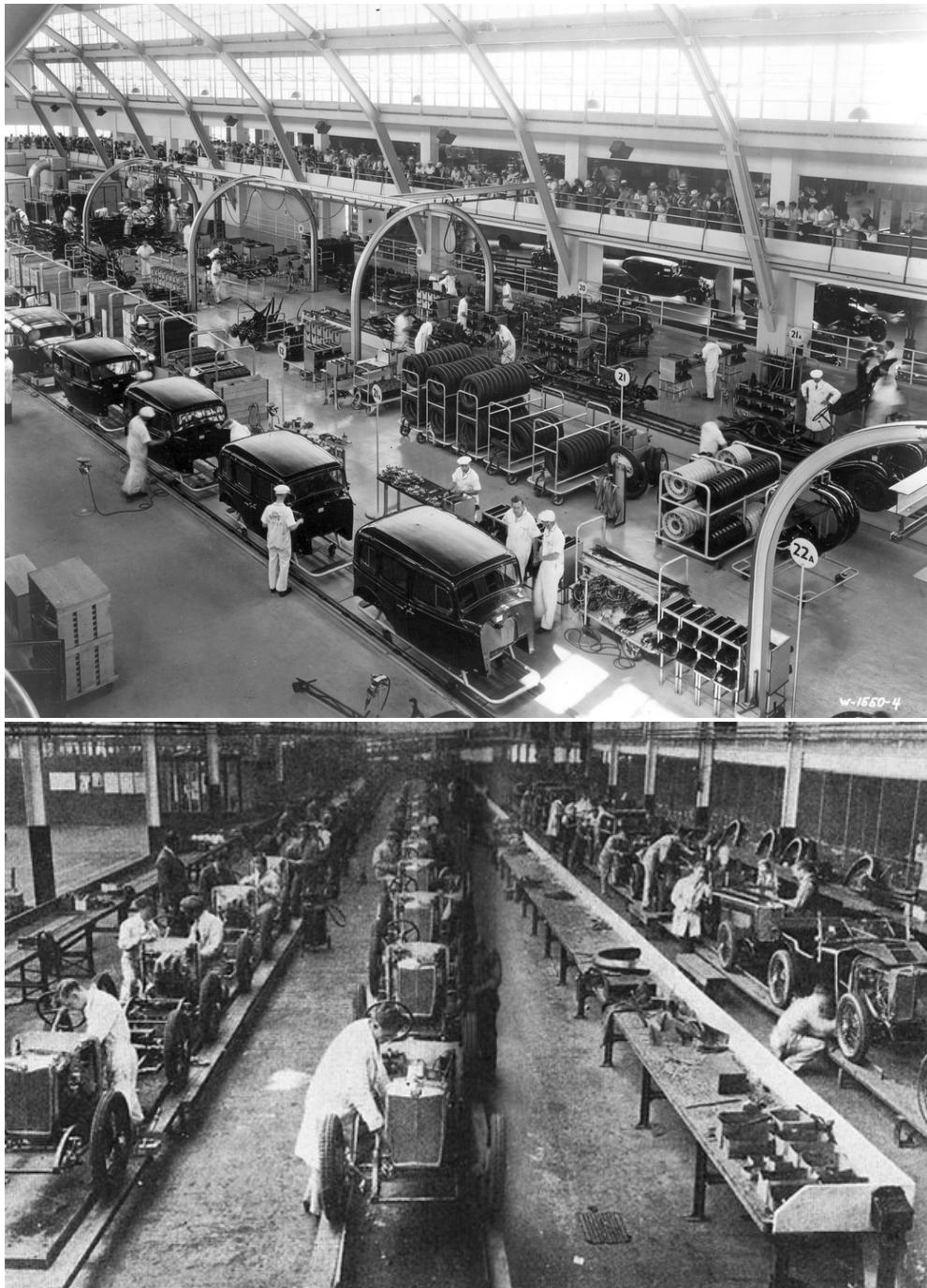
Figure 2.3: Early 20th-century Henry Ford's assembly line setup for the mass production of automobiles [20].
