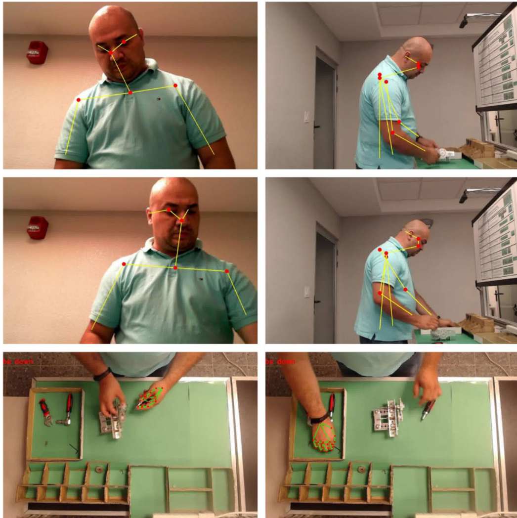
Figure 4.9: Example of hand detection and skeleton identification via imaging systems [87].
